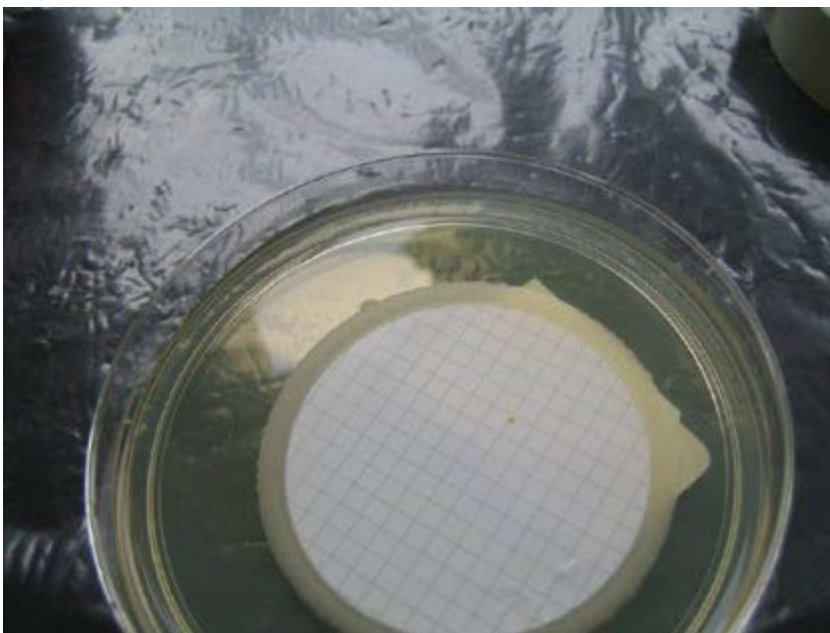
Fig. 7: Growth at the edge of the filter in membrane filtration: use of reusable material with insufficient sterilisation Source: VDMA Food Processing Machinery and Packaging Machinery
