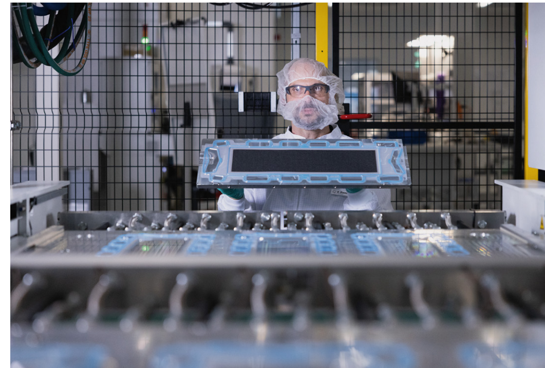
Die Membrane Electrode Assembly (MEA) wird unter Reinraumbedingungen hier bei Freudenberg e-Power Systems hergestellt. The Membrane Electrode Assembly (MEA) is manufactured under clean room conditions here at Freudenberg e-Power Systems. Quelle/Source: Freudenberg e-Power Systems
